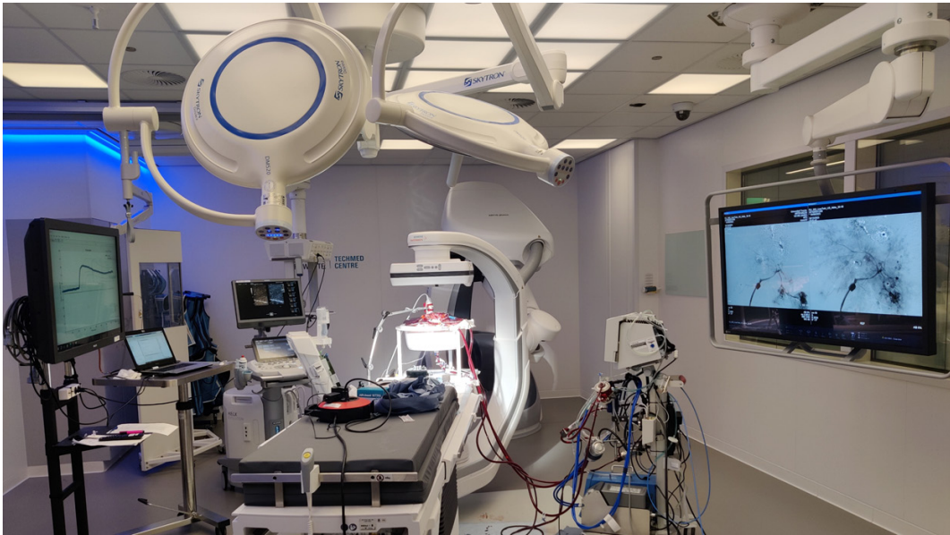
Figure 1. Overview of the experimental setup for development of the DCE-US radioembolisation protocol. From left to right: a) a display showing the analysed ultrasound data in TICs for multiple injection locations, b) an ACUSON S2000 ultrasound system showing both a contrast mode and a B-mode image, c) a perfused porcine liver on top of the reservoir including a 9L4 ultrasound transducer, d) the in-house developed perfusion apparatus for normothermic oxygenated blood perfusion of a porcine liver, e) X-ray images for microcatheter guidance using a digital subtraction angiography (DSA).
