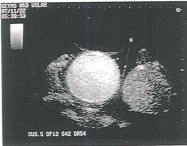
Fig.2a B-mode image of the ferrite micropowder suspension in mildly viscous fluid (=x5 diluted Aquasonic®). Right (darker) ball is mirror ghost of the left (brighter) one, due to vessel wall.
