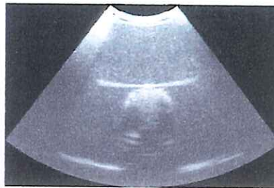
Figure 3: Demodulated image after optimized 1-tap filtering. Dynamic range: 55 dB.
