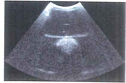
Figure 5: Demodulated image after optimized 64-tap filtering. Dynamic range: 55 dB.
